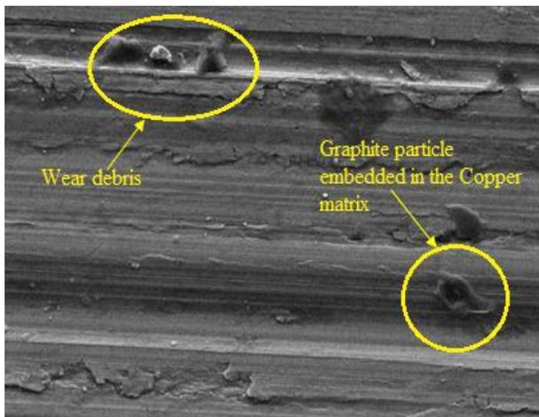
Fig 1: SEM analysis of MMC with 15% graphite and 30 N load (500x). [9]
