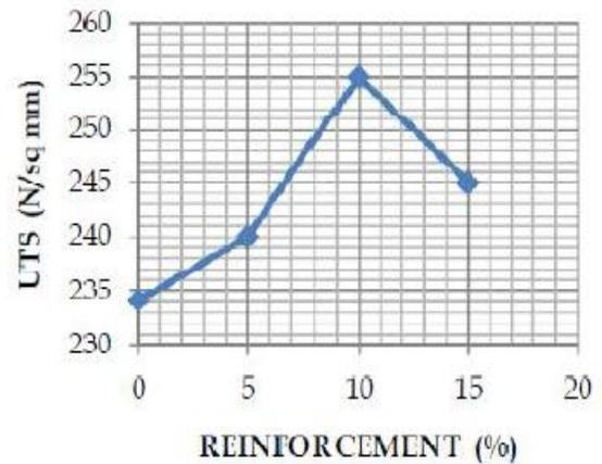
Fig 3: Ultimate tensile strength curve for different combinations of reinforcement [16]
