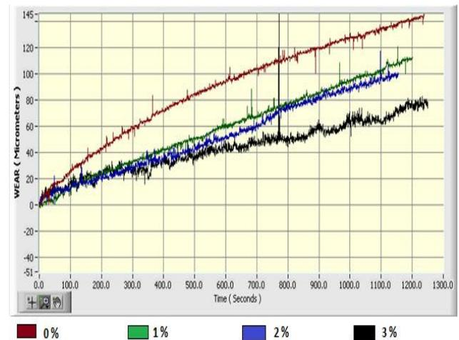
Fig 2: Wear behaviour of Al+ZrO<sub>2</sub> composite [13]
