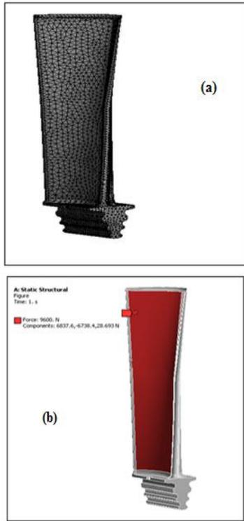
Figure 3: Meshed view of steam turbine blade
