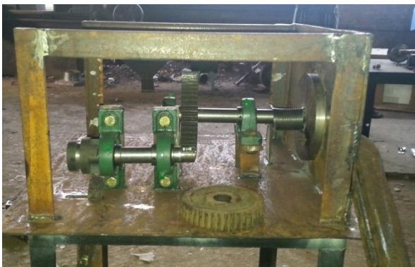
Figure 7: Front & Side View of HPFM for stirrup making machine
