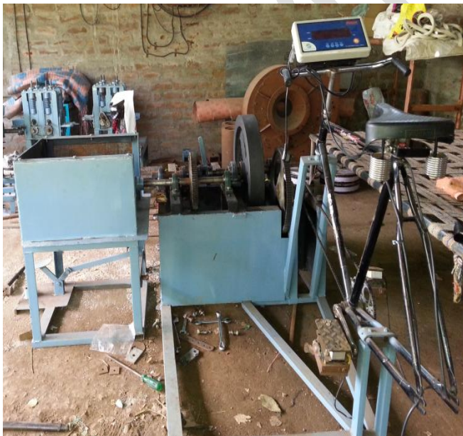
Figure 5: Fabricated View of human energized flywheel motor for stirrup making machine
