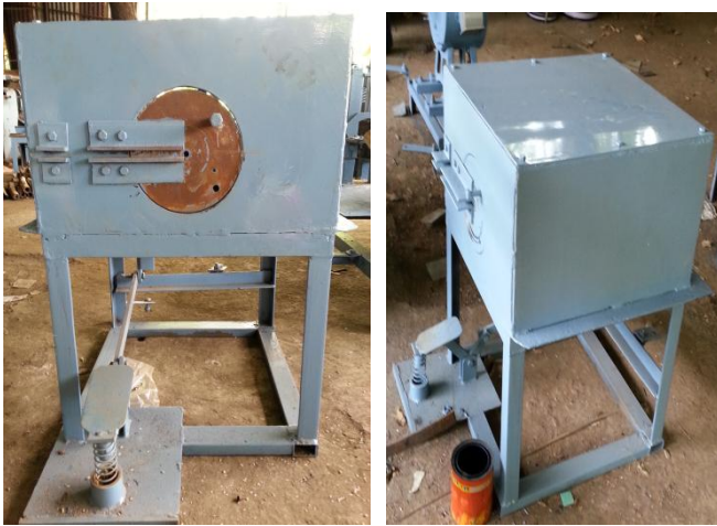
Figure 7: Front & Side View of HPFM for stirrup making machine
