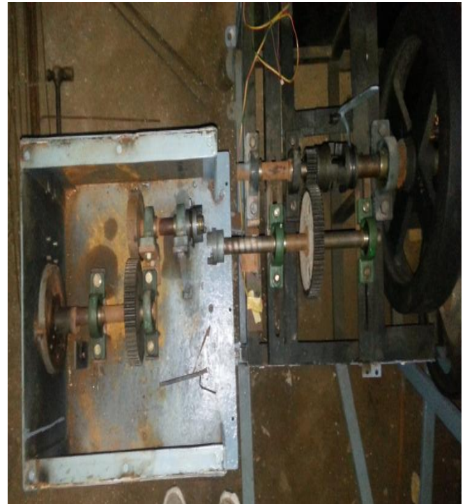
Figure 6: Top View of human energized flywheel motor for stirrup making
