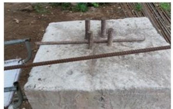
Figure 2. Concrete block as a platform for stirrup making
