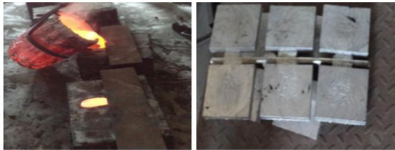
Fig.4 Pouring of Prepared Composite in Mould and Obtained Casting
