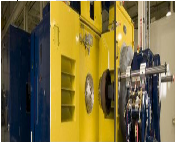
Fig. 18 NVH brake testing bench
