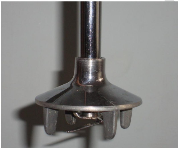
Figure 1.3: actual photograph of shaft of homogenizer used for steering mixture
