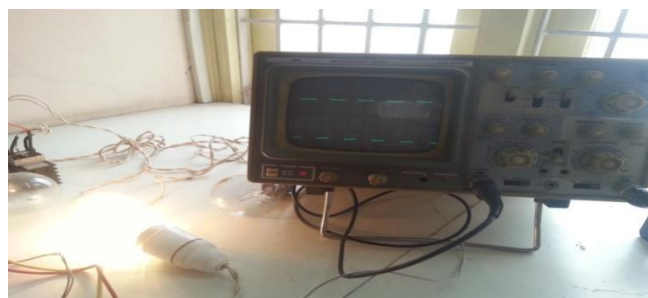
Fig.8: CRO output for 50% duty cycle with incandescent bulb
