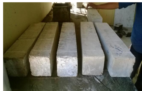
Fig.6 curing of specimens (self curing)
