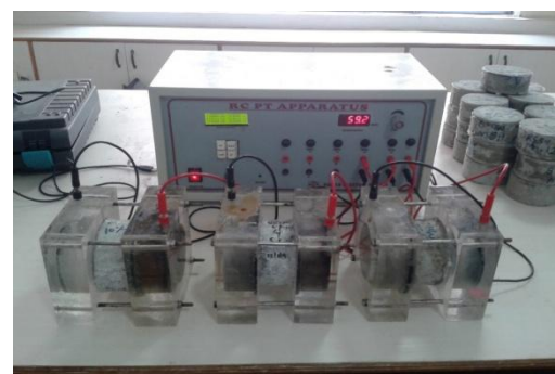
Fig. 8 Rapid chloride permeability test apparatus
