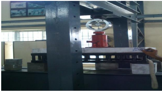
Fig. 9 deflection test for slab
