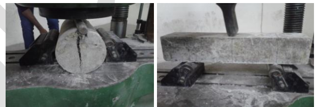
Fig. 7. Cylinders and Beams during testing
