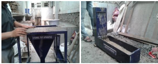
Fig. 1. Conductance of V-funnel and L-box test
