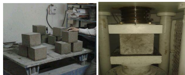
Fig. 2. Cubes before and during testing under CTM
