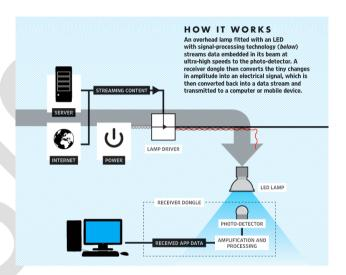
Radio frequency communication requires radio circuits, antennas and complex receivers, whereas Li-Fi is much simpler and uses direct modulation methods similar to those used in low-cost infra-red communications devices such as remote control units. Infra-red communication is limited in power due to eye safety requirements, whereas LED light bulbs have high intensities and can achieve very large data rates.
