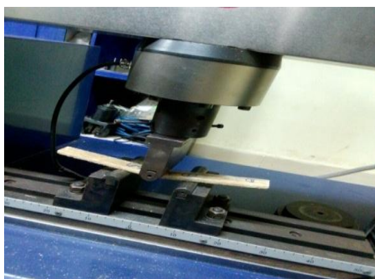
Fig.7. Specimen for Flexural test
