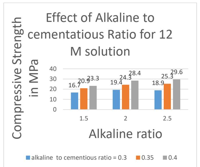
Figure 3: Compressive strength of AAC for 12 M solution.
