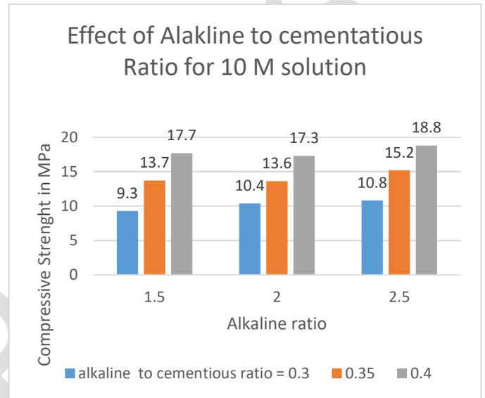
Figure 2: Compressive Strength for 10 M solution
