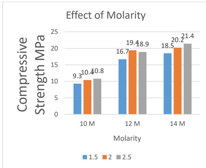
Figure 4: Compressive strength of AAC for different Molarity.
