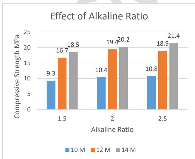
Figure 5: Comparative results of AAC with different
