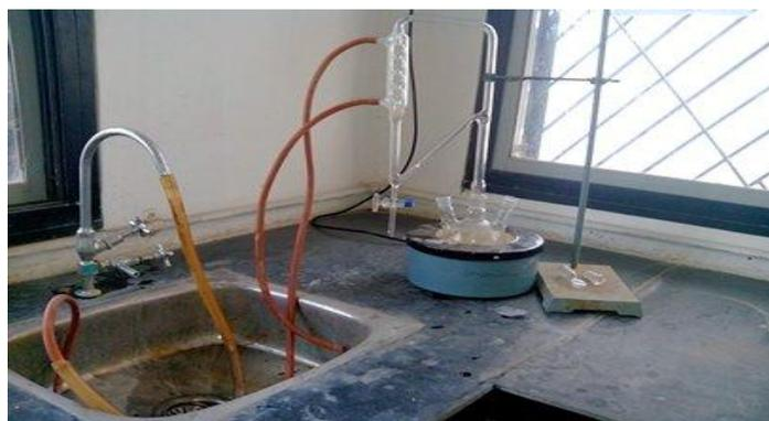
Clevanger apparatus [1] consists of a steam generator connected to the round bottom flask through a glass inlet tube. The flask is connected to a water condenser through a glass outlet tube. Condenser is further attached to a receiver through an adaptor.
