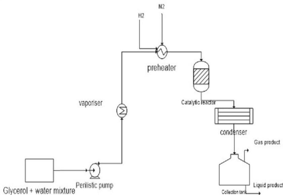
Fig.1. Schematic of glycerol steam reforming setup
