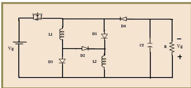
Fig. 6 Switched Inductor Buck Boost Converter
