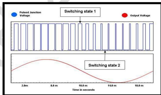
Fig. 12 Unipolar (Two Level) Switching Scheme
