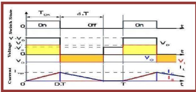
Fig. 5 Current and voltage waveforms in discontinuous mode
