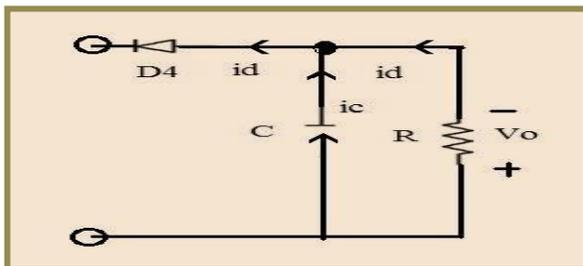
Fig. 9 Current flows through Diode D<sub>4</sub>
