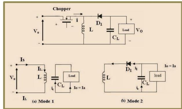
Fig. 3 Circuit diagrams of Buck Boost converter, Mode 1 and Mode 2
