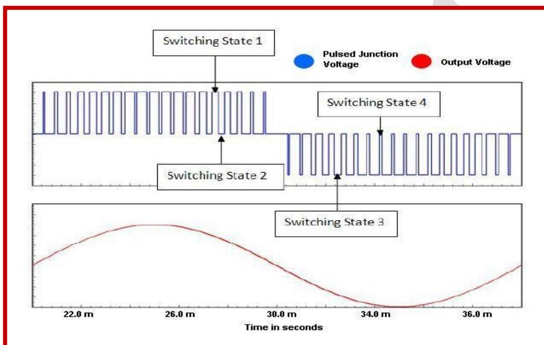
Fig. 14 Unipolar (Four Level) Switching Scheme
