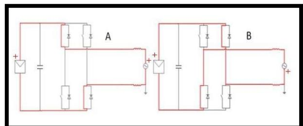
Fig. 13 A-Current Path for Full Bridge Converter implementing Bipolar Switching Scheme during Switching State-1, B-Current Path for Full Bridge Converter implementing Bipolar Switching Scheme during Switching State-2
