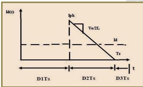
Fig. 8 Diode D<sub>4</sub> Current
