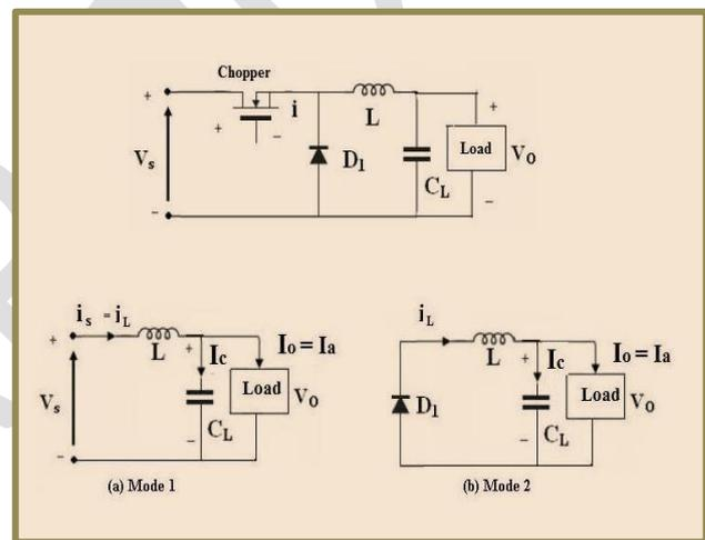
Fig. 1 Circuit diagrams of Buck Converter, (a) Mode 1 and (b) Mode 2
