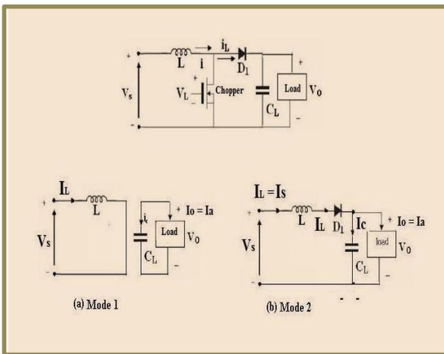
Fig. 2 Circuit diagrams of Boost converter, (a) Mode 1 and (b) Mode 2
