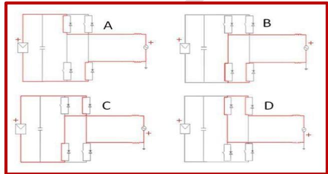
Fig. 15 A-Current Path for Full Bridge Converter implementing Unipolar Switching Scheme
