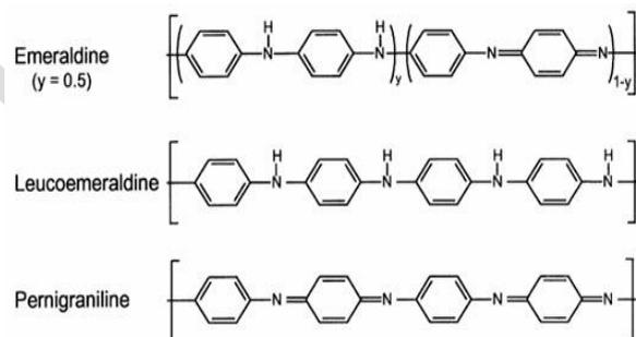
Fig: 1. Three oxidation states of Polyaniline
