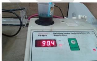
Fig.5 Conductivity Test of polyaniline
