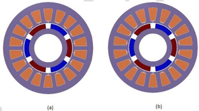
Fig. 2 (a) 14.9 mm stator slot depth (b) 15.9 mm stator slot depth
