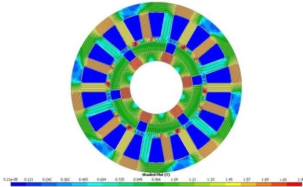
Fig. 4 Instantaneous field plot of 70 W radial flux motor for 15.9 mm stator slot depth
