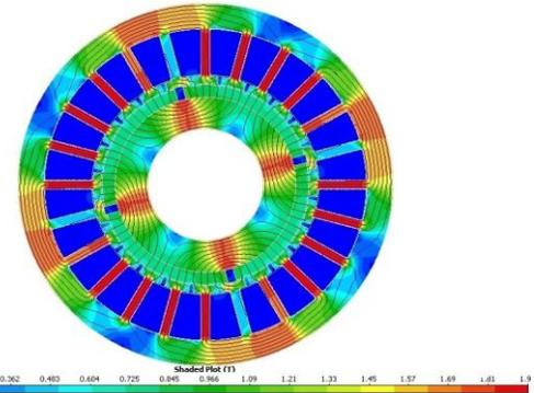
Fig. 7 Instantaneous field plot of 2.2 kW radial flux motor for 22.4 mm stator slot depth
