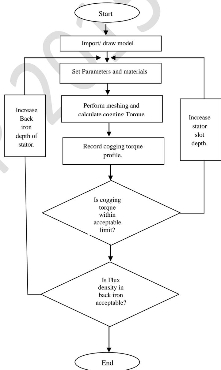
Fig. 1 Simulation step of cogging torque calculation
