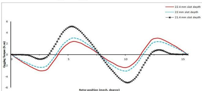
Fig. 6 Cogging Torque profile of 2.2 kW radial flux motor
