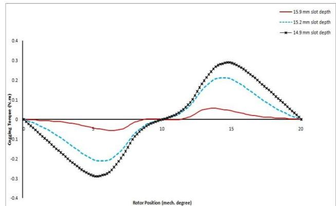
Fig. 3 Cogging Torque profile of 70 W radial flux motor
