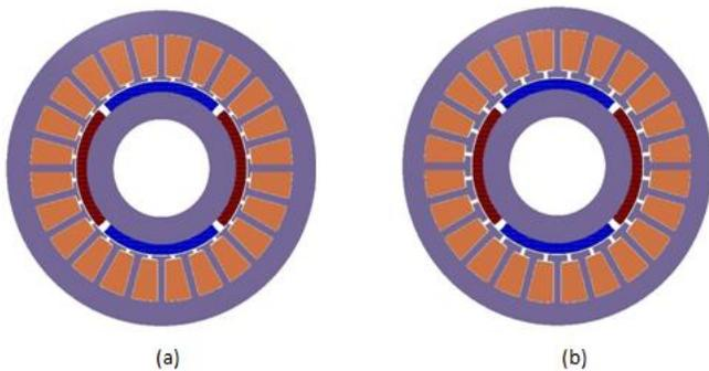
Fig. 5 (a) 21.4 mm stator slot depth (b) 22.4 mm stator slot depth
