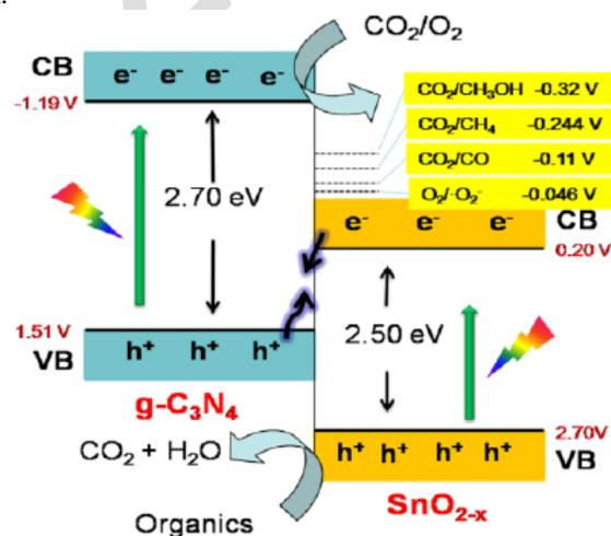
Figure 1 Z-scheme mechanism of SnO<sub>2</sub>/g-C<sub>3</sub>N<sub>4</sub>[2]
