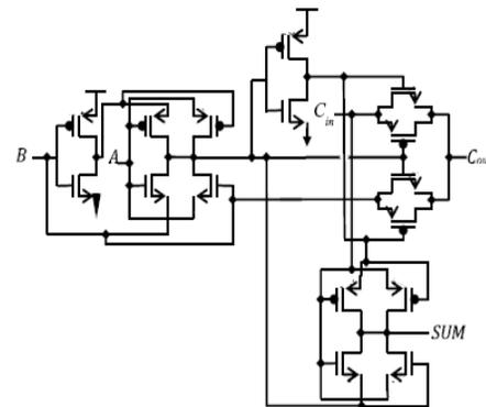
Fig.5 Hybrid CMOS2 full adder [4]
