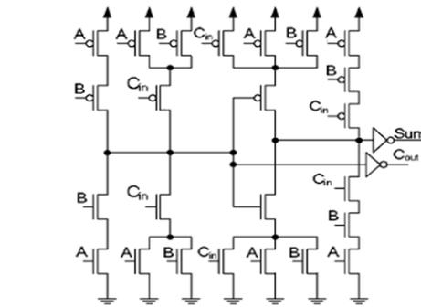
Fig.3 28T Mirror CMOS full adder [3]
