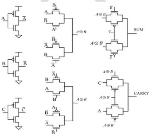
Fig.2 Hybrid CMOS1 full adder [6]
