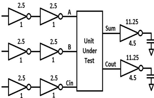
Fig.8 Test bed used for Simulation [7]
