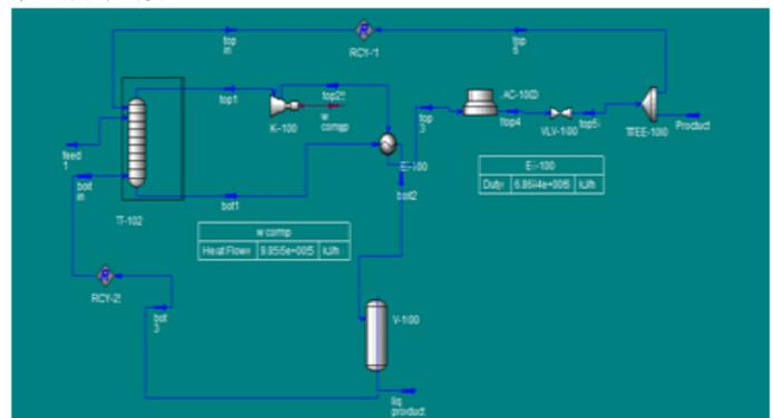
Fig. 2 Hysys process flow diagram for the vapour re-compression heat pump
