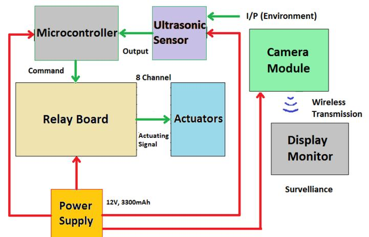
Fig.3: Block diagram of Electronic Circuitry
