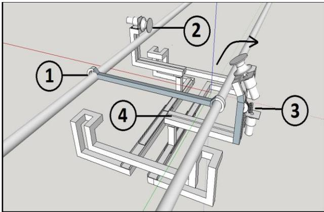
Fig.2: 1. Spacer, 2. U-Grooved Wheel, 3. Gear Assembly, 4. Main Chassis [8]
