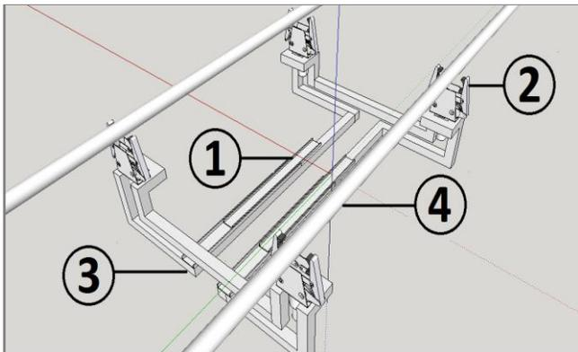
Fig.2: 2. Telescopic Slider, 2. Gripper Module, 3. Support Chassis, 4. HV Line [8]
