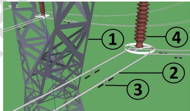
Fig.1: 1. Tower, 2. Bundled Conductors, 3. Suspension Clamps, 4. Vertical String Insulators [8]
