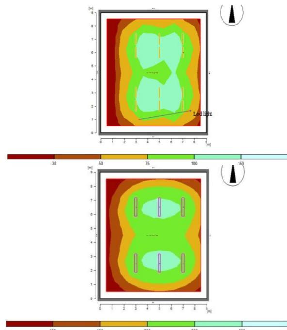
Fig. 2 Comparison between LED Light Effect in 9x 9 m Room (First Image) and 36 W Fluorescent Tubelight in 9x9 Room (Second Image) as generated by Relux
