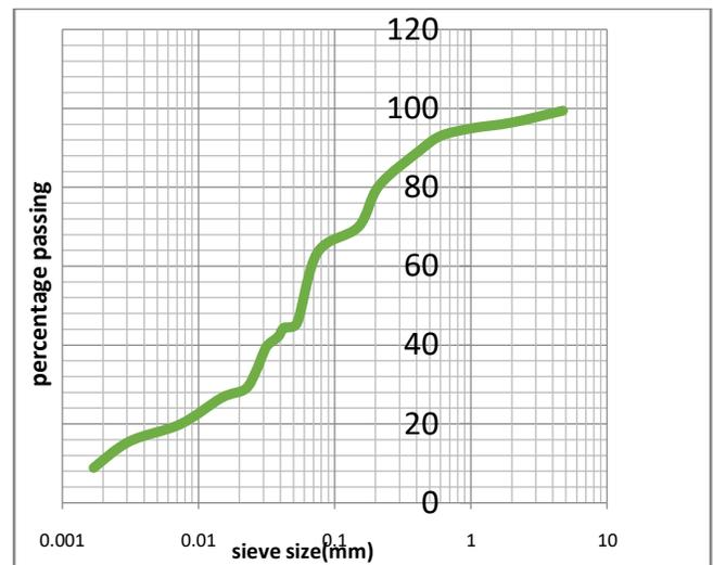
Figure: 2 Grain size distribution curve of natural soil
