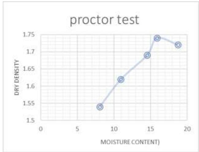
Figure 1: standard proctor test
