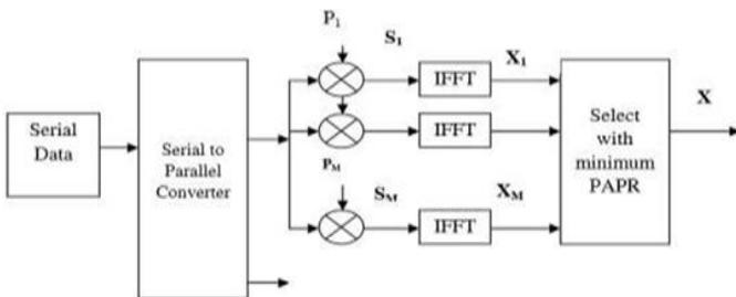
Fig.2. Block diagram of Selective Level Mapping
