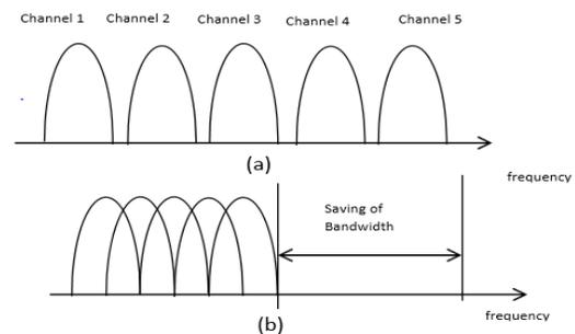
**Fig.1.** Comparison of (a) conventional multi-carrier technique and orthogonal multi-carrier modulation technique
