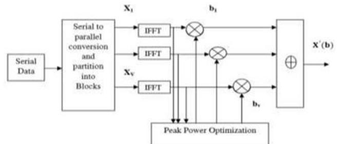
Fig.3. Block diagram of Partial Transmit Sequence
